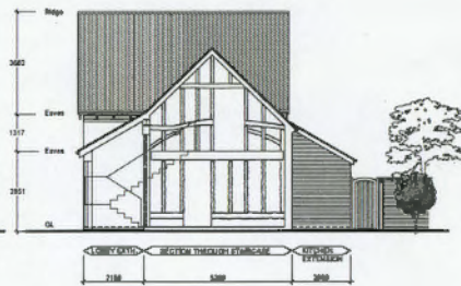
PROPOSED NORTH EAST ELEVATION OF RESULT BUILDING
